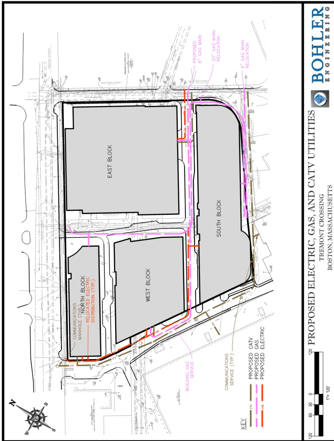
Figure 6-4: Proposed Electric, Gas and CATV Utilities
