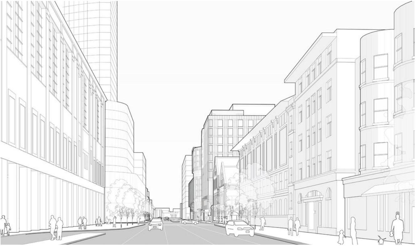
Eastern Approach along Boylston. The softly shifting form of the proposal appears as multiple buildings to break down the scale of the block between Mass Ave and Hereford Street. A regular pattern of openings relates to the traditional mixed use fabric along Boylston Street in the Back Bay.
