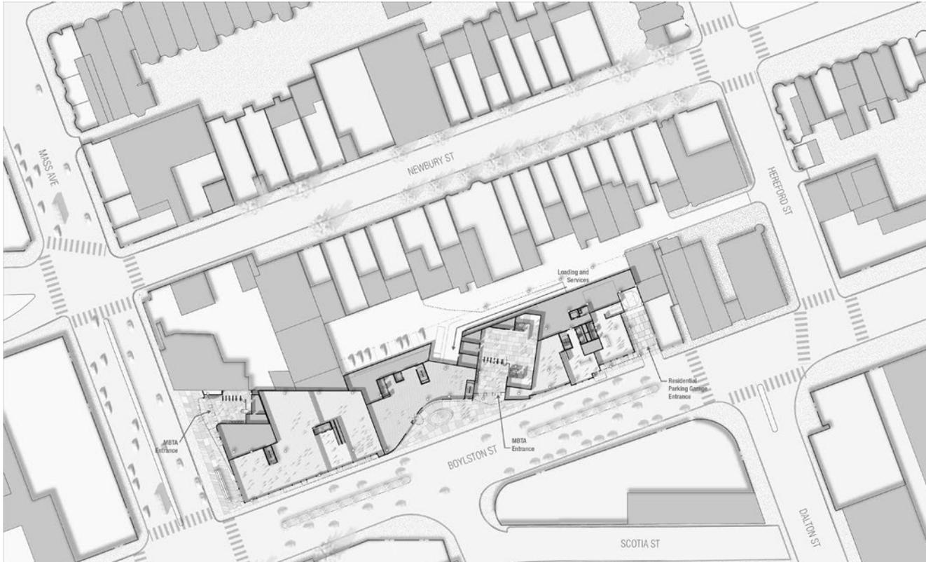
Ground Level Site Plan. The Viola reacts to the surrounding urban pressures to responsibly fill out the block between Mass Ave and Hereford Street. The ground plane of the new public plazas extends into the MBTA stations along both Mass Ave and Boylston Street opening the block to active, public uses through all seasons, with a diverse mix of retail, public transit, hotel and residential uses that will keep the new urban magnet energetic across the daytime and into the evening.
