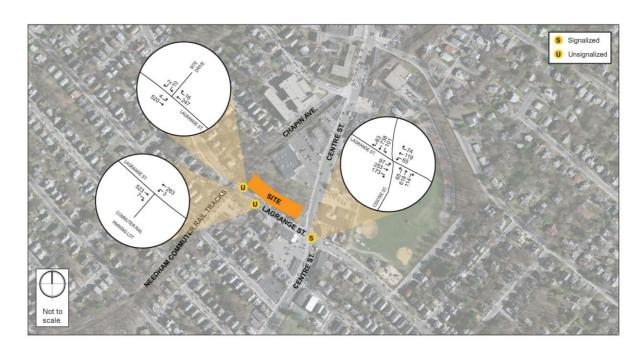
Figure 2-15 Build Conditions (2019) Turning Movement Volumes, p.m. Peak Hour
