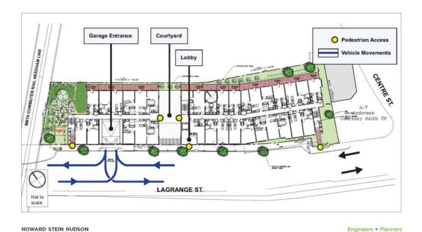
Figure 2-10 Site Access Plan – Garage Level
