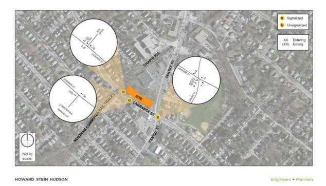
Figure 2-14 Build Conditions (2019) Turning Movement Volumes, a.m. Peak Hour
